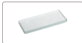
50mm reading scale (check magnification accuracy)
